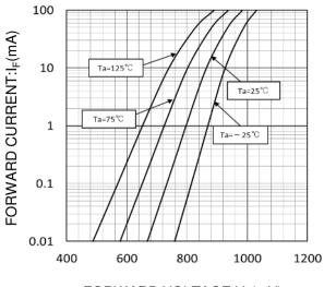
$\begin{array}{l} {\sf FORWARD\ VOLTAGE:} V_{\sf F}({\sf mV}) \\ V_{\sf F}\text{-}I_{\sf F}\ {\sf CHARACTERISTICS} \end{array}$
