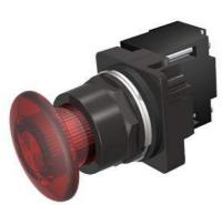
30mm BlackMax, Epoxy Coated Corrosion Resistant Complete Metal Unit Illuminated Push-Pull Operator Transformer type, 240V AC Incandescent Lamp Mushroom Head Cap Small 1 3/4" (44.5 mm) Plastic, Red 2 Position Maintained, Pull-to-Release UL Listed, CSA Certified NEMA 1,3,3R,4,4X,12,13 & Automotive Standards
