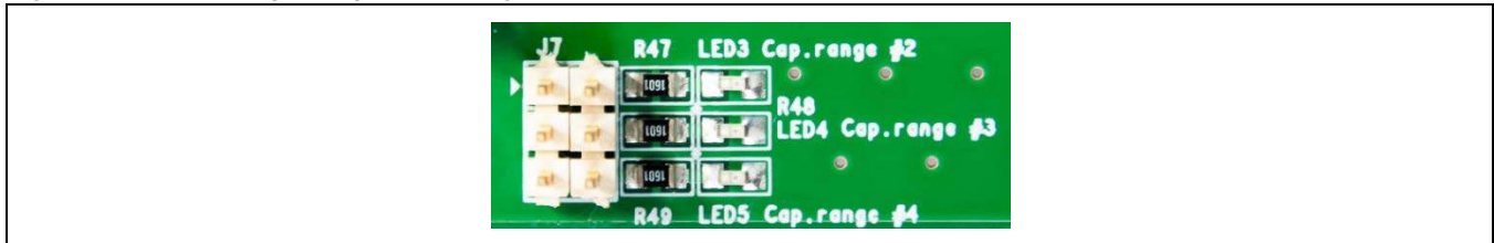
Figure 6.1 J7 - Output Capacitor Range Hardware Selection
