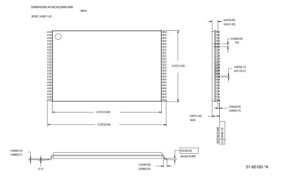
48-pin TSOP I (12 x 18.4 x 1mm) (51-85183)
