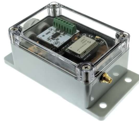
Pic. 22. Beehive LoRa monitoring system
