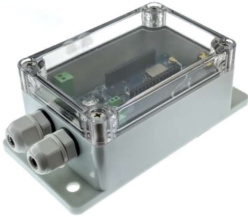
Pic.8. qBox Enclosure Kit with Arduino MKR Compatible (AMC) board installed
