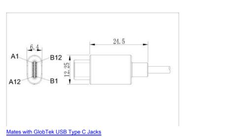
This cable includes a 22K pullup resistor between the 'CC' line and ' $V_{BUS}$ '. For systems compliant with the USB Type-C Cable and Connector Specification, the cable current will be restricted to 1.5A.
