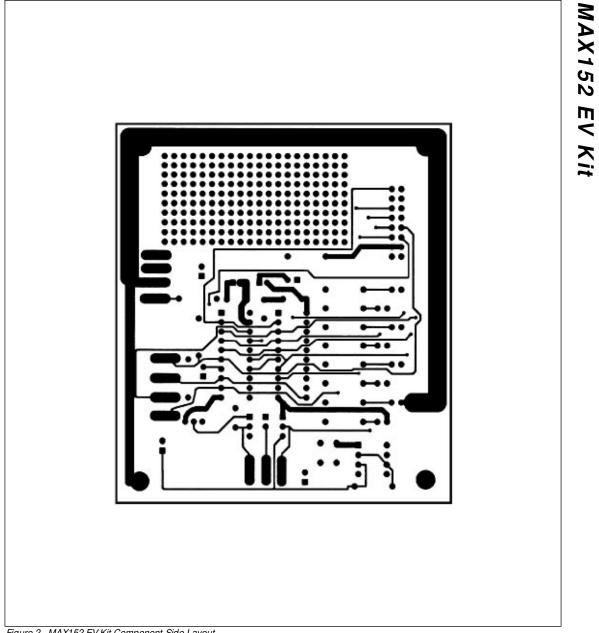
Figure 2. MAX152 EV Kit Component-Side Layout
