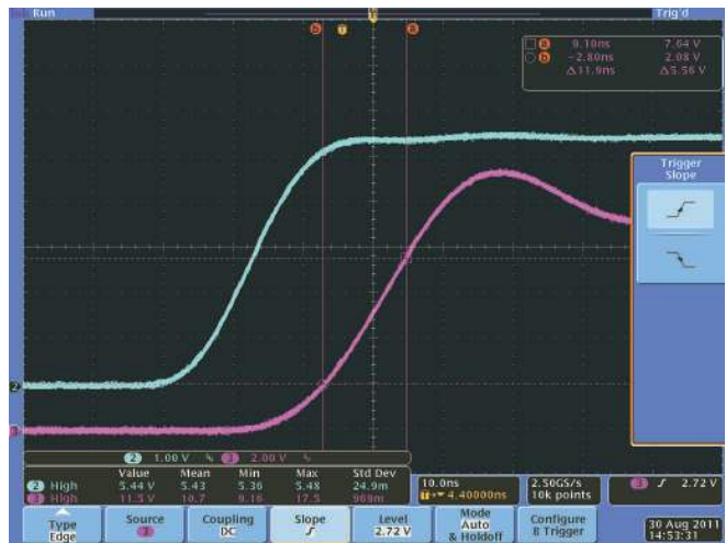
Figure 26. Typical Turn-Off Waveform (VDD = 10 V, C L = 1 nF)
