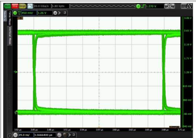
Figure 21. Eye Diagram at 4 Mbps PRBS 2^{16} - 1 , 2.5 V and 25°C
