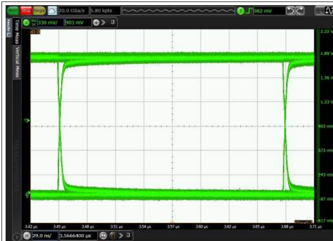
Figure 20. Eye Diagram at 4 Mbps PRBS 2^{16} - 1 , 1.8 V and 25°C
