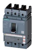
circuit breaker 3VA5 UL frame 250 breaking capacity class H 65kA @ 480V 3-pole, line protection TM230, FTAM, In=80A overload protection Ir=80A fixed short-circuit protection Ii=5...10 x In UL 489 SB (naval), 50 °C without connection
