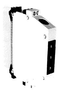
KSG 173 (3T) fitted with a pre-selector switch VS 632. The switch units are mounted one above another and can be snapped into the cable housing to lock in place. The dimensions of the switch units exactly match those of the opening in the cable housing so that no modification to the KSG 173 necessary.
