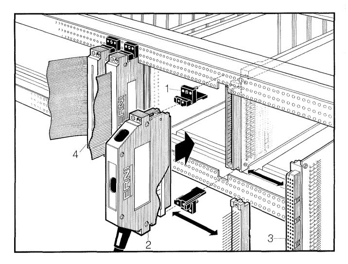
In a similar way to front-mounted connectors, this interface system also provides for making mateable interconnections directly from the wiring field to a printed circuit board. The guide elements are mounted on the rails of a subrack and serve to locate the PCB in the rack.
