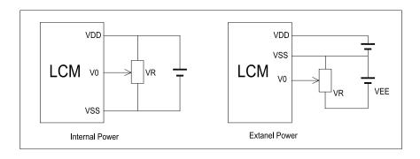
VDD~V0: LCD Driving voltage
