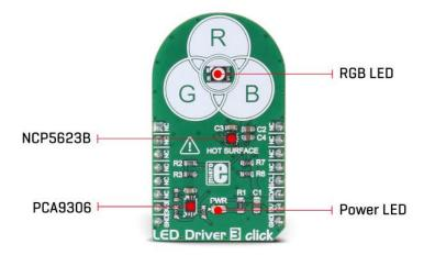
The gradual dimming function allows an easy way of dimming RGB LED intensity. With a simple I2C command, it is possible to trigger either upward or downward dimming. Dimming will affect the current through the LED segments, but the internal current limiter takes care not to exceed the maximum allowed current, set by the onboard resistor.
