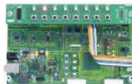
OM13320 Fm+ Demonstration Kit which includes the OM13260 Fm+ Development Board with two OM13303 GPIO Target Boards and one each of the the OM13399 Bridge and OM13401 PCA9617A bus buffer daughter boards
