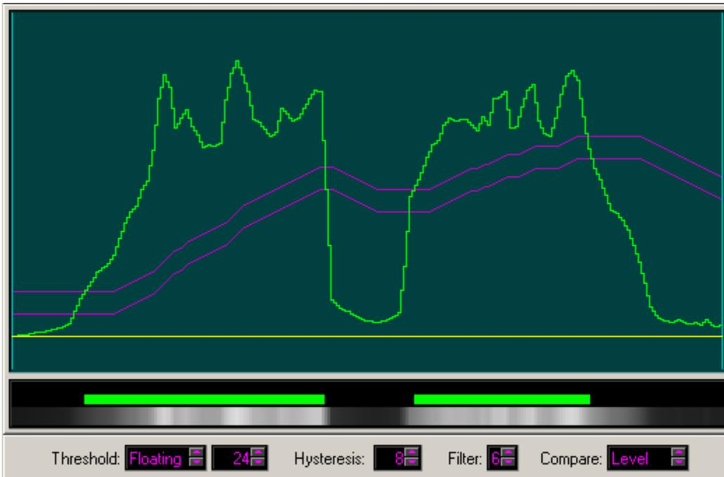
Here, a floating threshold with a filter factor of **6** has been selected. Now, see what happens when the filter factor is changed to **2**:
