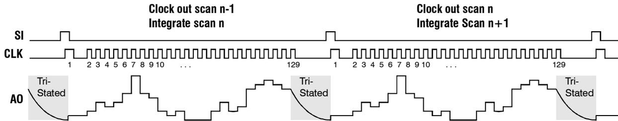
In one-shot imaging, the TSL1401R is left idle until it's time to snap a picture. Then **SI** clocked in, and 128 pixels are rapidly clocked out and discarded. Then you simply wait until the desired exposure time (since the **SI** pulse) has elapsed and pulse **SI** again. At this point, you can clock out the pixels resulting from the timed exposure. Here is a sample waveform:
