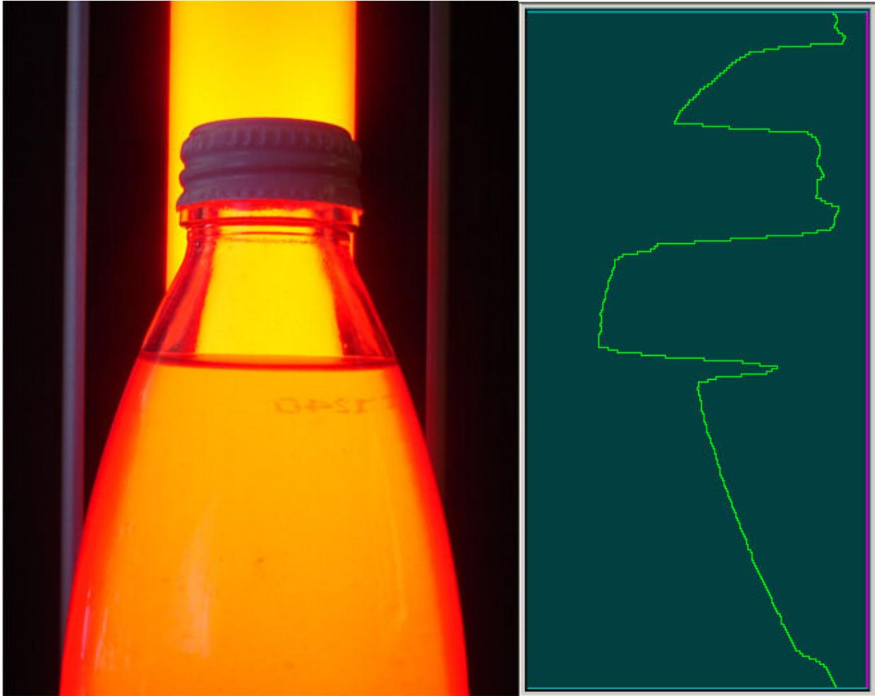
Clearly visible are the shadows created by both the cap and the meniscus at the liquid level. Although the juice in this example is colored, such a sharp meniscus will be present even with water-clear liquids. By measuring both the position of the meniscus and the size of the cap shadow, we can determine if the bottle is filled and capped properly.
