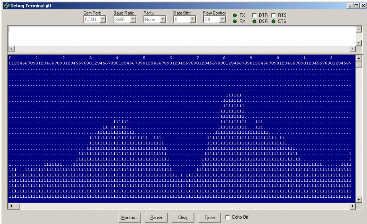
You can see where the hole is, as well as the outside edges. However, this also illustrates a couple pitfalls of front lighting: specular reflection (glare) from the black background surface (i.e. black not being all that black), and rounded-off edges. Proper lighting techniques encompass an entire subject area of their own. The last chapter of this document links to various resources on the internet that cover this important topic.
