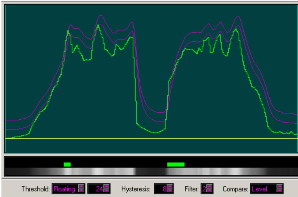
Only the most extreme rising edges are detected in this case, as indicated by the green area in the narrow strip below the scope window. In fact, one of the most important applications of floating thresholds is edge detection.
