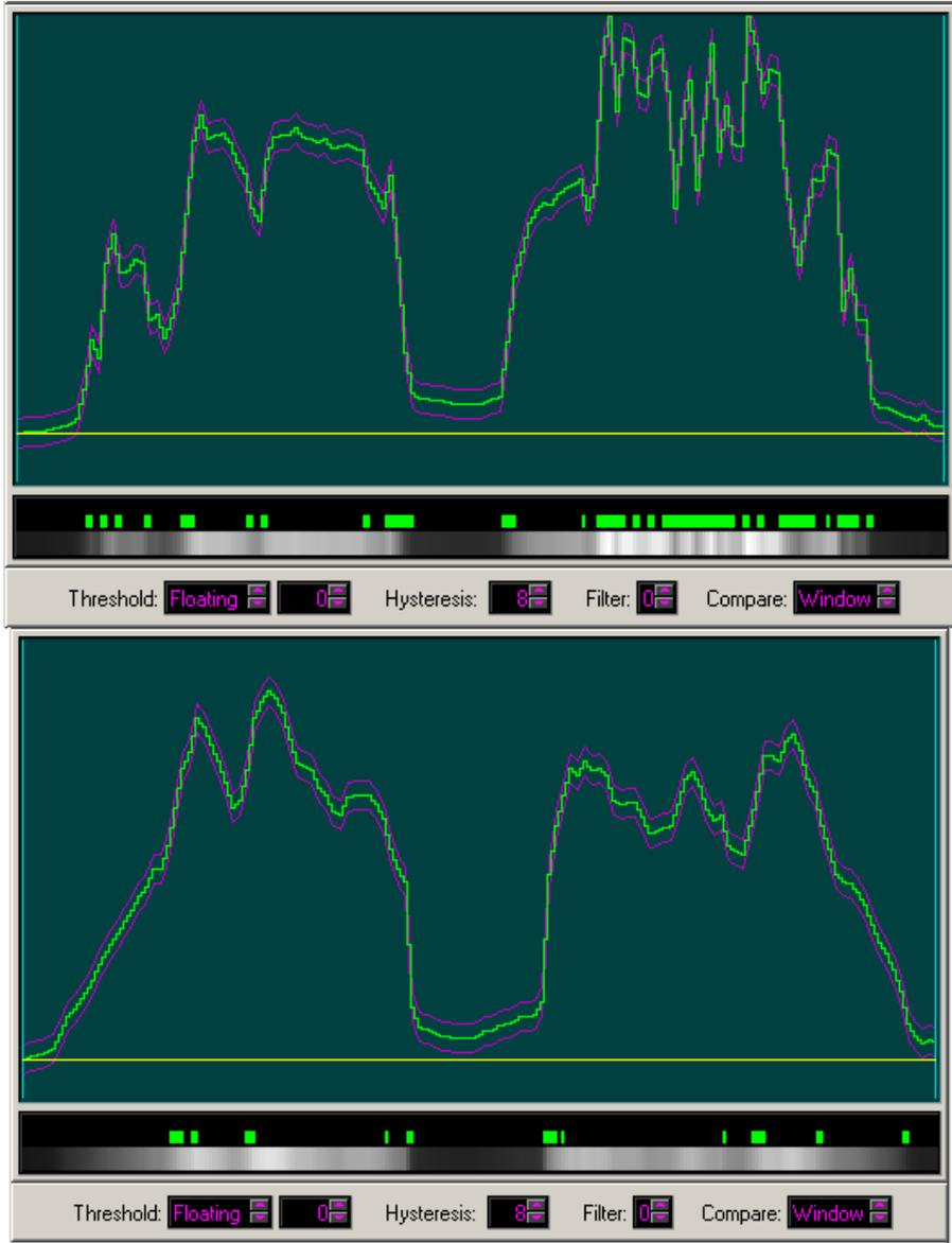
Notice how the green “one” pixels capture the texture of the coated bagel, and even the fact that the right side of that bagel has more stuff on it than the left side.
