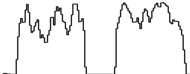
Here, you can see not only the edges of the bagel and the hole in the middle, but also the intensity variations caused by the seeds and herbs on its surface.
