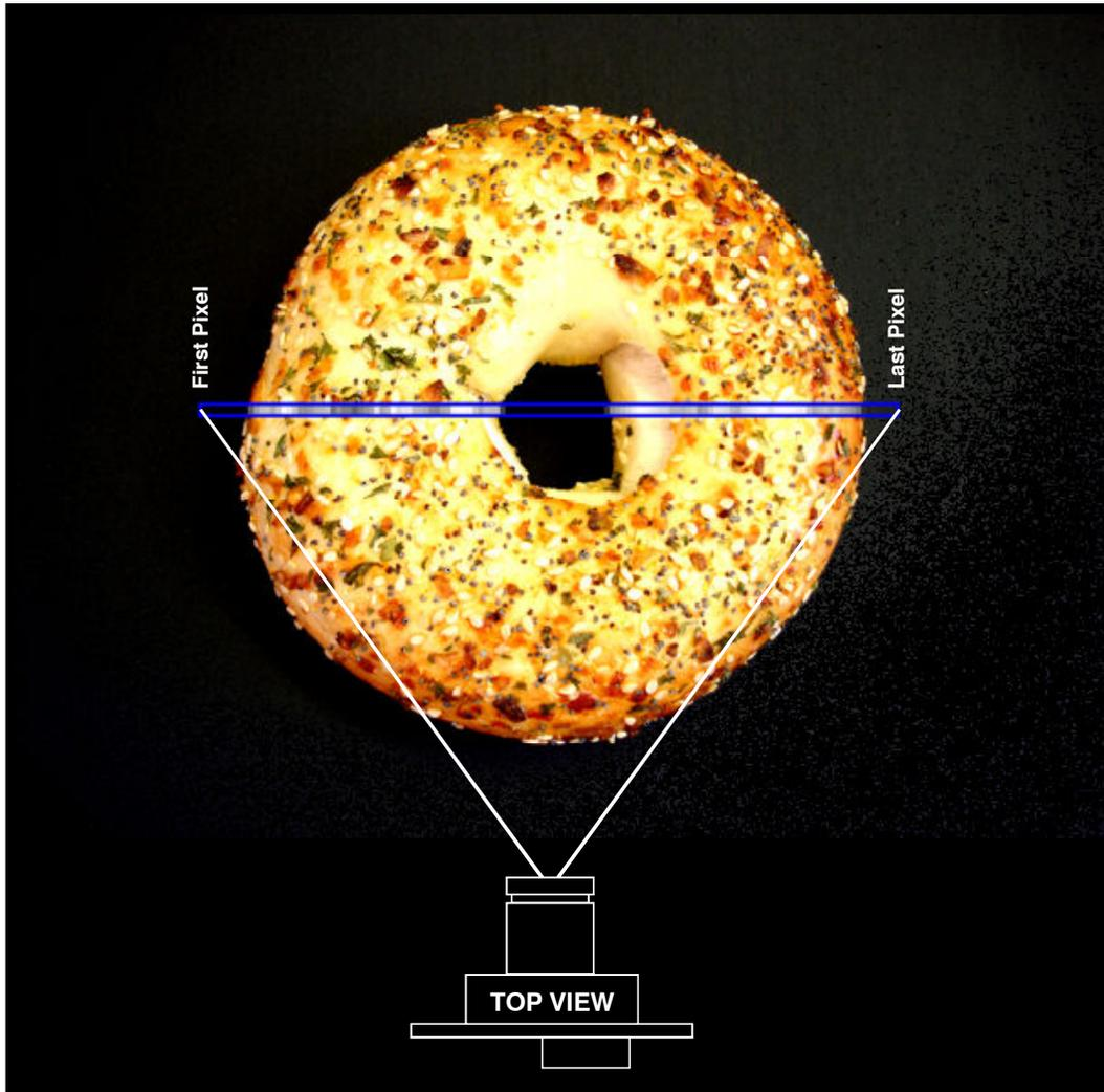
The output from each observed pixel is an analog voltage proportional to light intensity. The analog intensity curve corresponding to the image above would look something like this:
