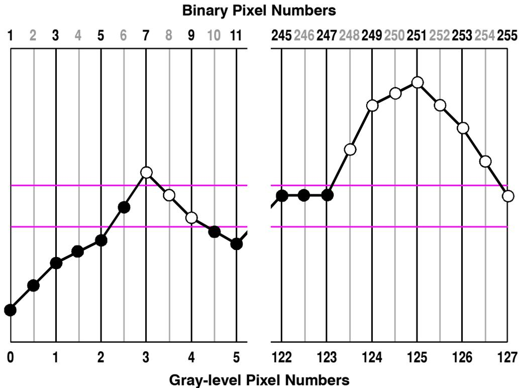
All light/dark thresholding takes place using the values of the 255 real and interpolated pixels, yielding 255 bits of data, whose positions are numbered **1** through **255**. (Note: This one-based numbering is different from that of the direct BS2 numbering shown earlier. That was zero-based to conform with PBASIC's zero-based subscript conventions.) Binary pixel **0** is non-existent in this system and is used in the context of image analysis to indicate "feature not found".
