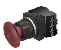
30mm BlackMax, Epoxy Coated Corrosion Resistant Complete Metal Unit Illuminated Twist-to-Release Transformer type, 600V AC Incandescent Lamp Mushroom Head Cap Small 1.79" (45 mm) Plastic Cap, Red 2 Position Maintained, Twist-to-Release with 1 N.O. - 1 N.C. Heavy Duty Contacts, A600/P600 UL Listed, CSA Certified NEMA 1,3,3R,4,4X,12,13 & Automotive Standards
