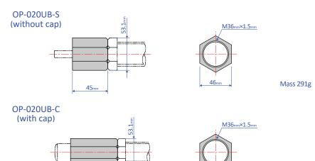
Note: When attaching, make sure that the side without a bearing chamfer is the impact surface.
