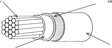
PRIMARY INSULATION - RADIATION-CROSSLINKED, MODIFIED PVDF COLOR - NATURAL PRIMARY JACKET - RADIATION-CROSSLINKED, MODIFIED ETFE
