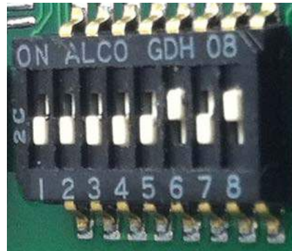
Master radio with DIP switches 6 and 8 in the ON position.
