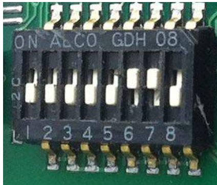
Slave radio with DIP switches 6 and 7 in the ON position.
