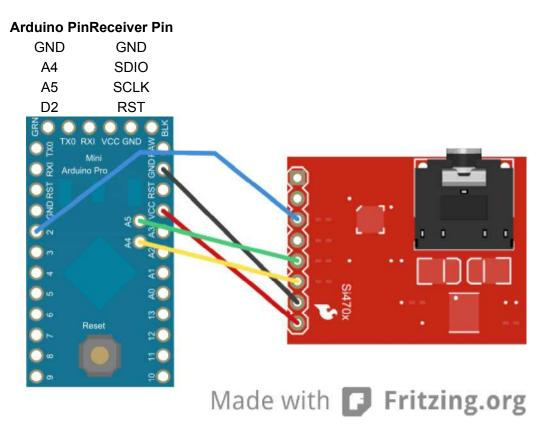
It's very important to realize that the Si4703 radio receiver breakout is a 3.3V device; that's why we're using an Arduino Mini Pro 3.3V. Using a 5 Volt Arduino (like the Arduino) can ruin the radio receiver if proper care isn't taken to shift the voltage levels down to an acceptable level. You can read this sensor interfacing tutorial to learn how to connect modules that communicate at different voltage levels.
