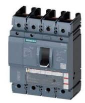
circuit breaker 3VA5 UL frame 250 breaking capacity class H 65kA @ 480V 4-pole, line protection TM210, FTFM, In=150A overload protection Ir=150A fixed short-circuit protection Ii=10 x In N conductor protection 100% without connection
