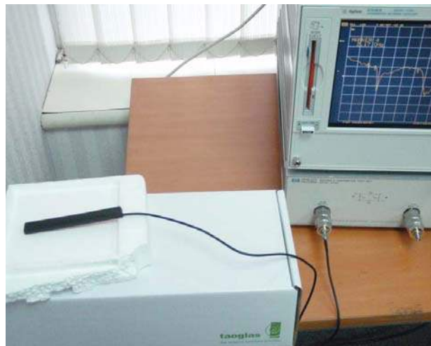
Free space Return Loss measurement setup
