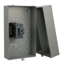
Electrically held lighting contactor, Contactor amp rating 100A, 0 N.C. / 3 N.O. Poles, 600VAC 60HZ coil, 1 NO / 1 NC auxiliary contacts Non-combination type, (no disconnect device), Enclosure NEMA type 1, Indoor general purpose use
