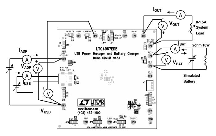
Figure 1. Proper Measurement Equipment Setup
