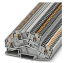
Double-level terminal block, with equipotential bonder, nom. voltage: 800 V, nominal current: 28 A, connection method: Push-in connection, 1st and 2nd level, cross section: 0.2 mm<sup>2</sup> - 6 mm<sup>2</sup>, mounting type: NS 35/7,5, NS 35/15, color: gray
