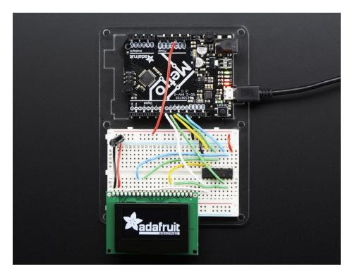
The power requirements depend a little on how much of the display is lit but on average the display uses about 50mA from the 3.3V supply. Built into the OLED driver is a simple switch-cap charge pump that turns 3.3V into a high voltage drive for the OLEDs.
