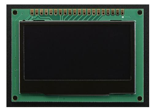
The pins on these modules are not well marked, but the one on left is #1 and the pins increment in order until the one on the very right, #20
