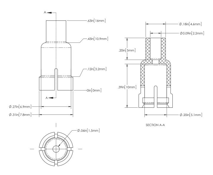
Standard Tolerance of ±0.005 inch / ±0.25 mm
