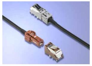
The MX79A Series are miniaturized high-speed automotive infotainment connectors designed to support data transmission. Speeds of up to 1.5 Gbps can be supported when used in conjunction with the MX55J Series of automotive camera connectors. Four mating key variations are available to prevent incorrect mating when multiple connections are used for the same module.
