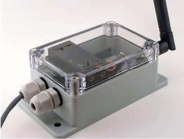
Pic. 18. 2xAAA battery holder applied to a transparent lid (assembled view)
