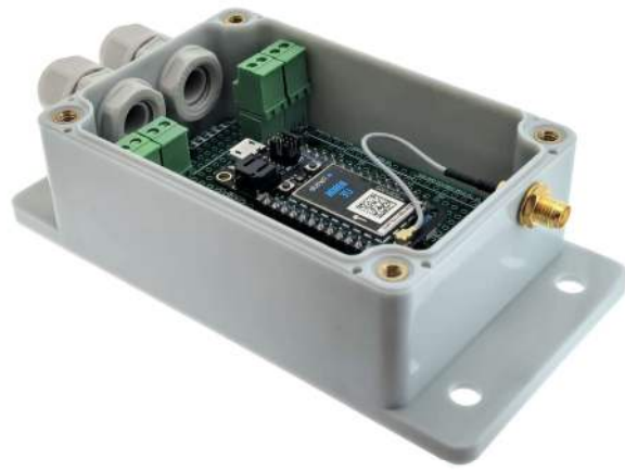
Pic.9. qBox AFC Enclosure Kit with Adafruit Feather Compatible (AFC) board installed
