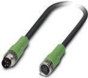
Sensor/Actuator cable, 4-position, PVC, Black RAL 9005, Plug straight M8, on Socket straight M8, Cable length: 5 m
