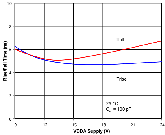
Figure 3.6. Rise/Fall Time vs. Supply Voltage
