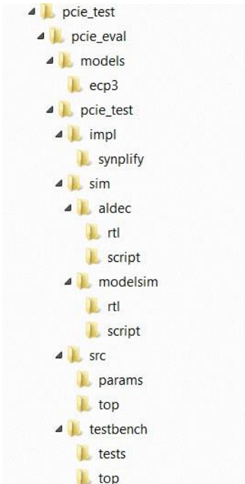
Figure 4.3. LatticeECP3 PCI Express Core Directory Structure
