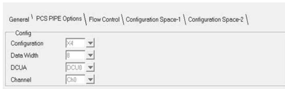
Figure 3.2. PCI Express IP Core PCS Pipe Options
