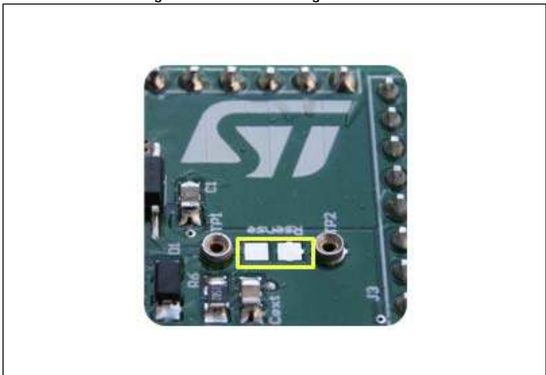
Figure 5. Pads for soldering SMD resistor
