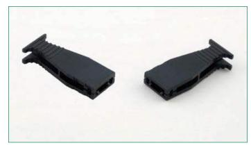
This fuse puller is designed to allow for easy removal of MINI<sup>®</sup> fuses and other MINI<sup>®</sup> style components. Its narrow profile enables you to remove a fuse even when nested between two larger components (i.e. relays.) The material used provides a robust design that lasts through multiple fuse withdrawal cycles.
