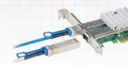
As virtualization, consolidation, and convergence initiatives continue to grow, so do the demands placed on the physical infrastructure. To meet the needs for faster processing speeds, low power server inter-connect and I/O consolidation deployments, Panduit offers 10Gig™ SFP+ Direct Attach Passive Copper Cable Assemblies.
