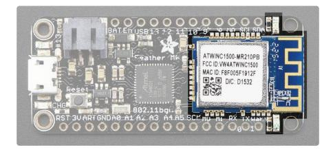
Since not all pins can be brought out to breakouts, due to the small size of the Feather, we use these to control the WiFi module
