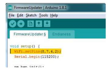
Upload it to your board. Make sure the Serial console is not open before or after uploading.
