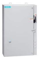
Non-reversing motor starter Size 3 Three phase full voltage Solid-state overload relay OLRelay amp range 25-100A 380-440/440-480V 50/60HZ coil Combination type 125Amp circuit breaker Enclosure NEMA type 4/12 Water/dust tight for outdoors Standard width enclosure
