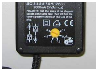
Figure 2-3: DC voltage selection
