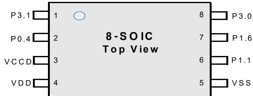
Figure 8. 8-Pin SOIC Pinout
