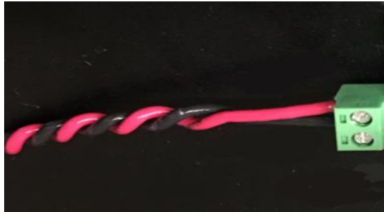
Figure 2. Example of Twisted Leads for Voltage Supply
