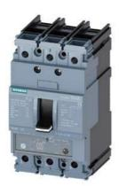
circuit breaker 3VA5 UL frame 125 breaking capacity class S 25kA @ 480 V 3-pole, line protection TM240, ATAM, In=50A overload protection Ir=40A ...50A short-circuit protection Ii=5...10 x In cable connection on both sides
