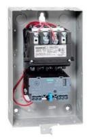
Non-reversing motor starter, Size 0, Three phase full voltage, Solid-state overload relay, OLRelay amp range 0.25-1a, 240V 50HZ / 277V 60HZ coil, Non-combination type, Enclosure type 12, Dust/drip proof for indoors, Standard width enclosure
