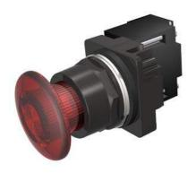
30mm BlackMax, Epoxy Coated Corrosion Resistant Complete Metal Unit Illuminated Push-Pull Operator Full Voltage, 6V AC LED Lamp Mushroom Head Cap Small 1 3/4" (44.5 mm) Plastic, Red 3 Position Momentary UL Listed, CSA Certified NEMA 1,3,3R,4,4X,12,13 & Automotive Standards
