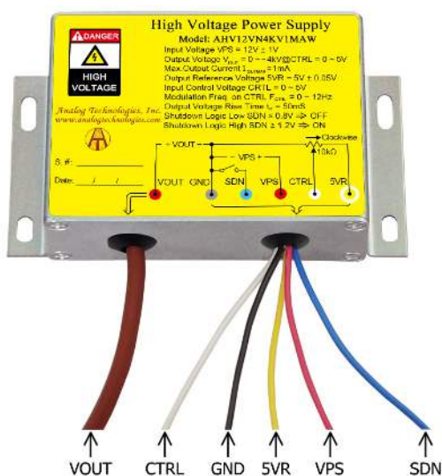
Figure 2. The Connecting Lead Wires of AHV12VN4KV1MA
