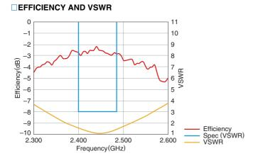
• Tested antenna has been soldered. Evaluation board size is 50x10x1 mm.
