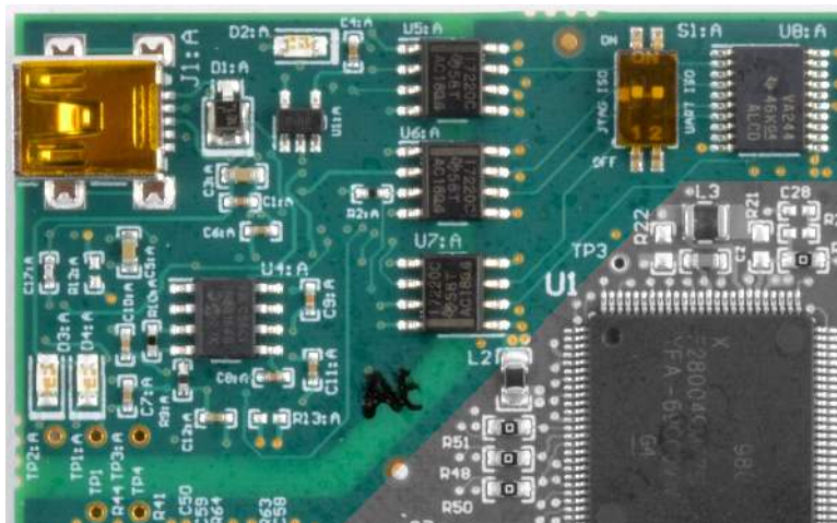
Figure 2. XDS100v2 Emulation Circuitry and Isolation Circuitry is Denoted by :A
