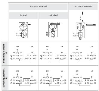
$<sup>\</sup>frac{1}{\mathbf{k}^{\prime}}$  Positive action N/C locking monitoring contact
