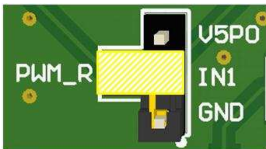
Figure 5. IN1 Connected to PWM Output
