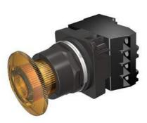
30mm BlackMax, Epoxy Coated Corrosion Resistant Complete Metal Unit Illuminated Twist-to-Release Transformer type, 120V AC LED Lamp Mushroom Head Cap Small 1.79" (45 mm) Plastic Cap, Amber 2 Position Maintained, Twistto-Release with 1 N.O. - 1 N.C. Heavy Duty Contacts, A600/P600 UL Listed, CSA Certified NEMA 1,3,3R,4,4X,12,13 & Automotive Standards
