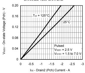
ON-STATE RESISTANCE (Pch) vs. CHANNEL TEMPERATURE
