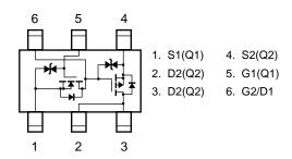
Remark The diode connected between the gate and source of the transistor serves as a protector against ESD.
